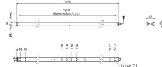
Mechanical InformationCasing MaterialAluminium + AcrylicWeight11kgOperating Temperature0°C to 40°C, Humidity 20%-85%Storage Temperature-20°C to 60°C, Humidity 20%-85%Lighting Dimension, W x L x H25.0 x 2230.0 x 55 mmIP RatingIP40
